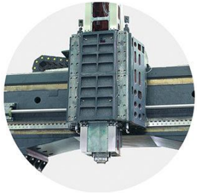
Square ram structure 500x500MM
